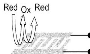
Fig. 4. Example of interdigitated electrodes for redox cycling (reproduced from reference [12]).
