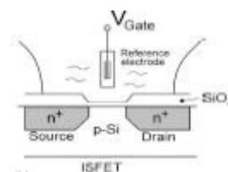
Fig. 7. Basic schematic structure of a n-type ISFET (reproduced from reference [16]).
