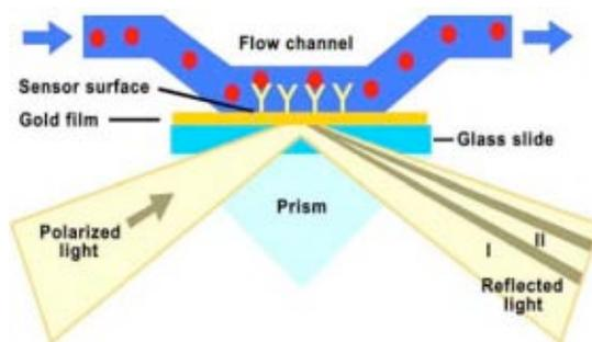
Fig. 3. Schematic setup of a SPR biosensor utilizing a flowcell structure (reproduced from reference [10]).
