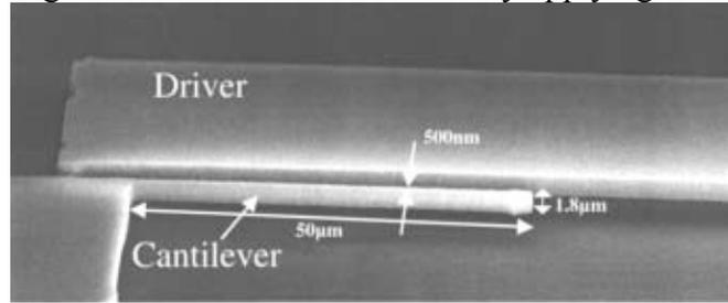
Fig. 1. SEM image of a working resonance cantilever detector (reproduced from reference [3]).
