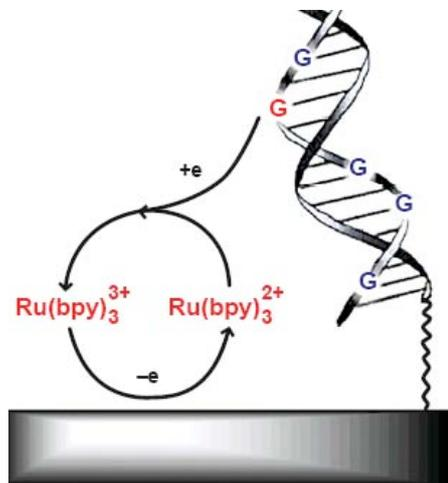
Fig. 5. Indirect detection of DNA through a redoxable molecule (Ru) (reproduced from reference [12]).
