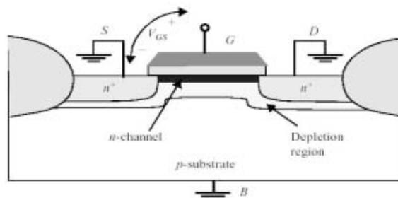
Fig. 6. Basic schematic structure of a n-type MOSFET (reproduced from reference [14]).
